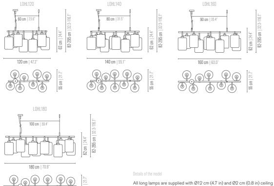
All long lamps are supplied with Ø12 cm (4.7 in) and Ø2 cm (0.8 in) ceiling covers HL-1, 250 cm (98.4 in) of double steel cable, and 350 cm (137.8 in) of electric cable. The total drop can be easily adjusted on-site.
